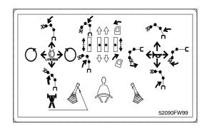
(18) **REFERENCE OPERATOR MANUAL** (Item 20) This warning label is positioned on the right side window of the cab.
